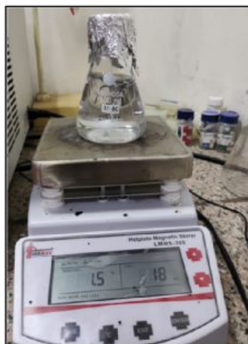
Fig 3.4: Determining the pH of plant and algal biochar
