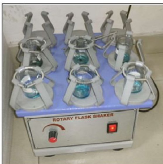
Fig 3.6: Test solutions put for continuous shaking on a mechanical shaker to assess remediation over time
