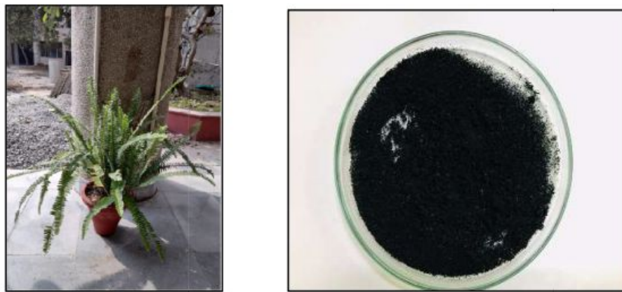
Fig 3.3: Synthesis of Nephrolepis auriculata biochar from dried plant leaves powder
