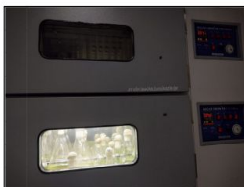
Fig 3.1: Microalgae cultured in BG-11 medium are incubated under optimum growth conditions in the algal growth chamber
