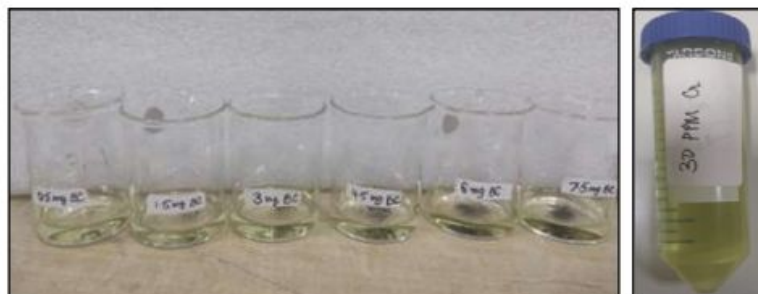
Fig 3.9: Test solutions containing varying concentrations of biochar
