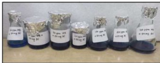
Fig 3.7: Test solutions for determining the effect of initial dye concentration on removal efficiency
