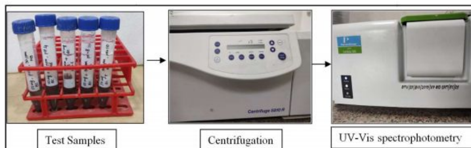
Fig 3.8: Procedure for calculating the removal efficiency of biochar
