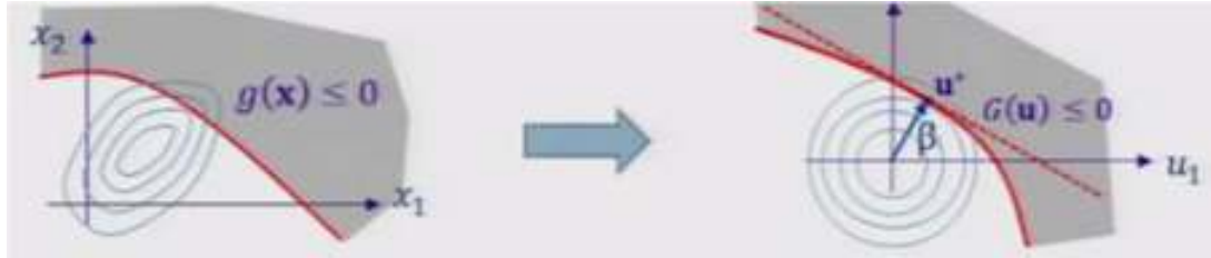
Fig 5.6 Reliability index and Design point representation
