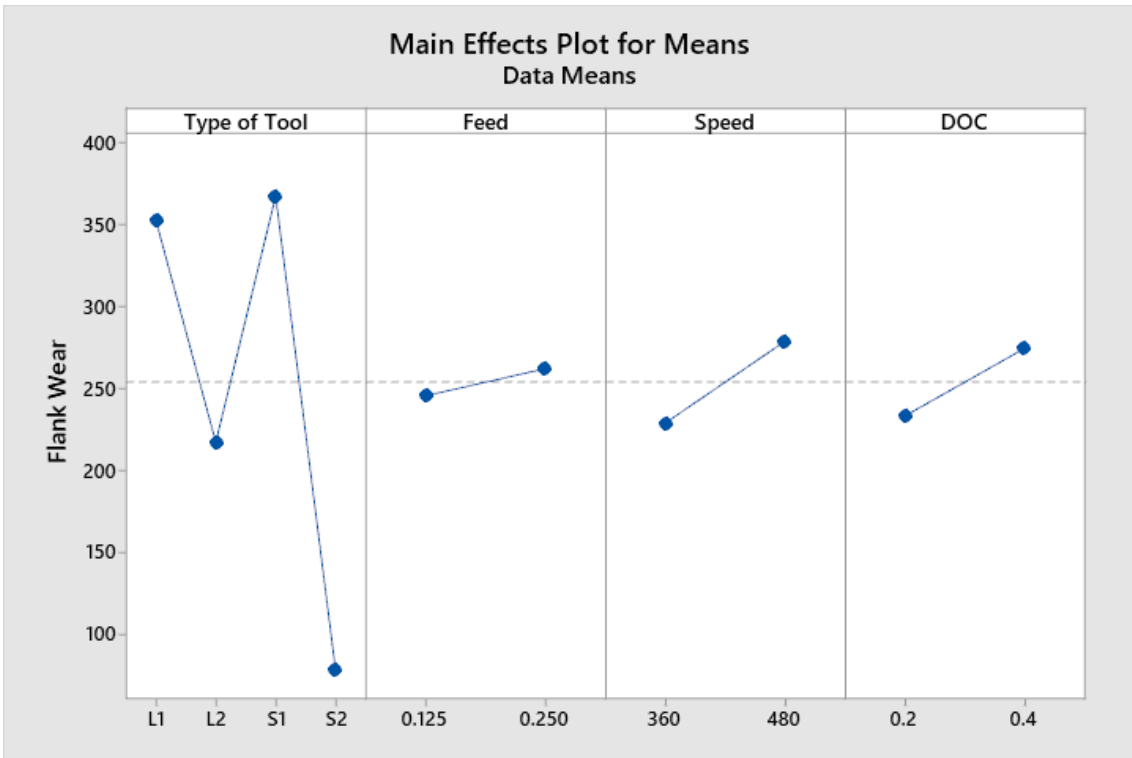
Figure 5.43: Effect plot of flank wear vs Type of Tool, Feed, Speed and DOC.
