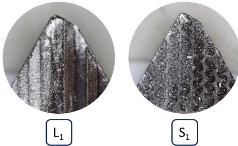
Figure 5.39: Microscopic images of the CNC tool inserts having Line and Sine Wave texturing perpendicular to the edge of the tool nose.
