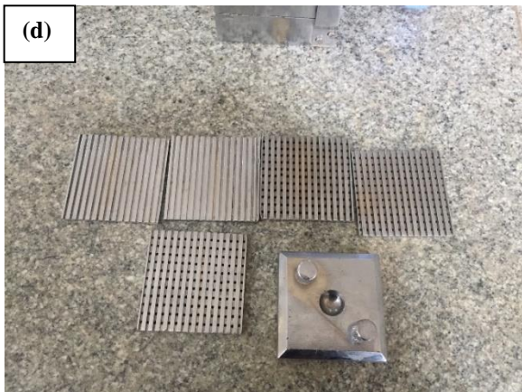
Fig. 3.4: (a) Direct Shear test apparatus (b) Shear box (c) Sample cutter and sample extractor (d) Grid plates and loading pad
