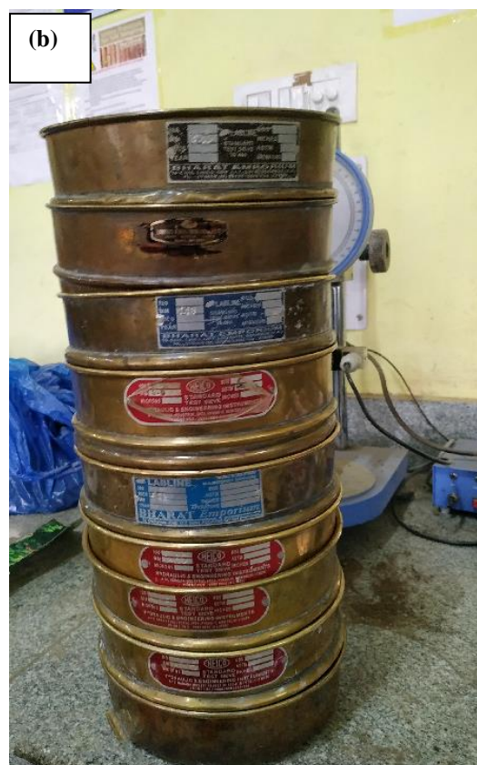
Fig. 3.1: (a) Soil fraction retained on 75 \mu IS sieve after wet sieving (b) Sieve arrangement for coarse sieve analysis.
