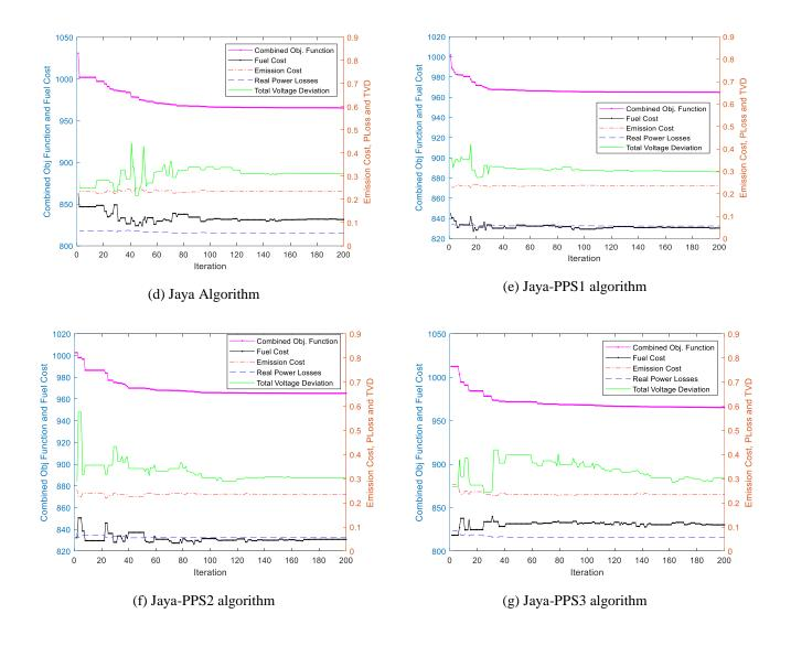
Fig. 7.2: Convergence and variation of objective functions, IEEE 30-bus system, Case 1
