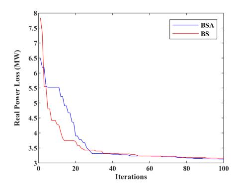
Fig 4.5: Convergence characteristics for IEEE 30-bus system, Case 5
