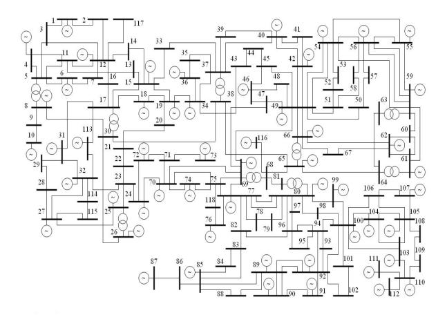
Figure D. Single line diagram of IEEE-118 Bus Test System
