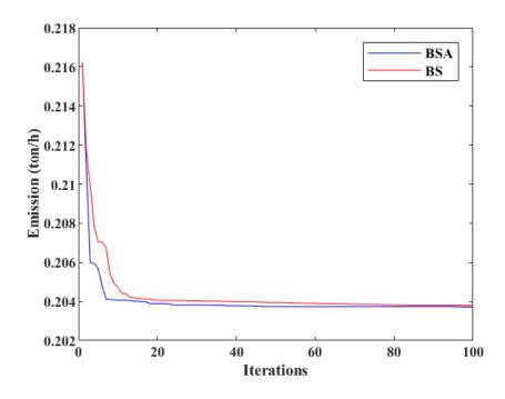
Fig 4.6: Convergence characteristics for IEEE 30-bus system, Case 6
