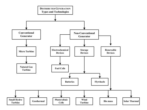
Fig 1.2: Types and technologies of distributed generation
