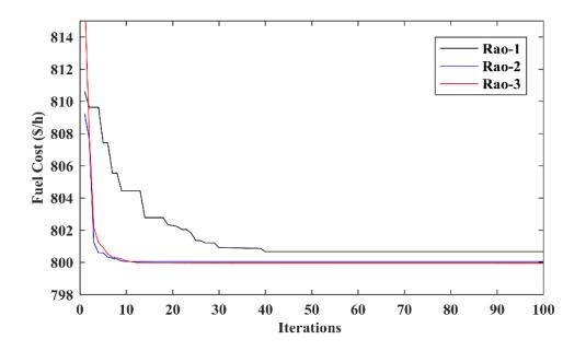
Fig 5.2: Convergence characteristics for IEEE 30-bus system, Case 1
