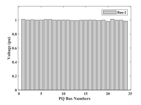
Fig. 5.3: Load bus voltage profile for IEEE 30-bus system, Case 2
