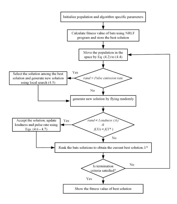
Fig. 4.1: Flowchart of bat search optimization algorithm
