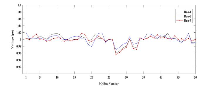
Fig. 5.7: Voltage profile at load buses in IEEE 57-bus system, Case 8
