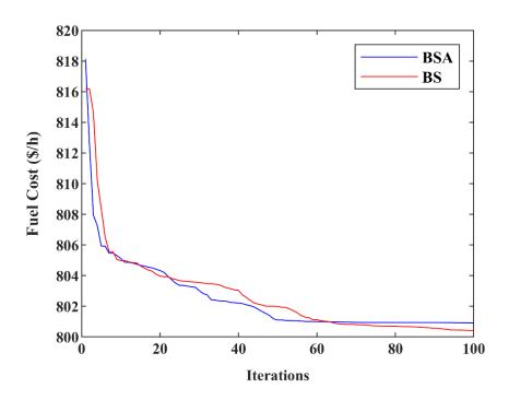
Fig 4.3: Convergence characteristics for IEEE 30-bus system, Case 1
