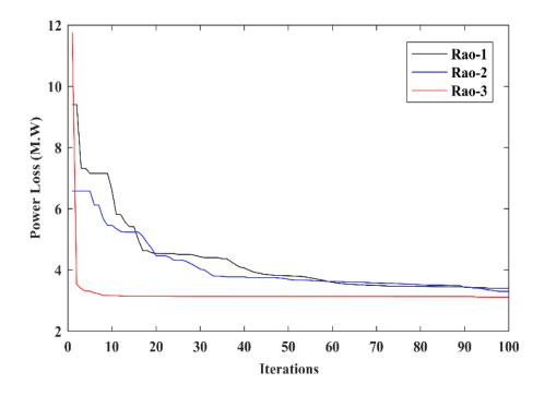
Fig. 5.4: Convergence characteristics for IEEE 30-bus system, Case 5
