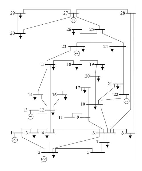
Figure A. Single line diagram of IEEE-30 Bus Test System
