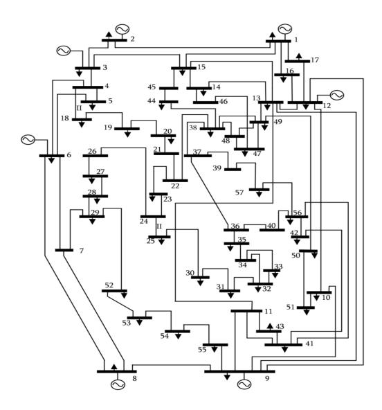
Figure B. Single line diagram of IEEE-57 Bus Test System
