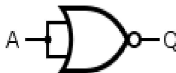
Fig 19. NOT Gate using NOR Gate
