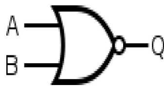
Fig 9. Symbol of NOR Gate
