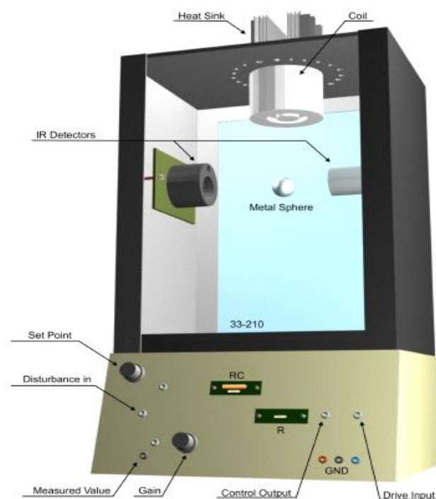
Fig 4.1 Feedback Magnetic Levitation System Model
