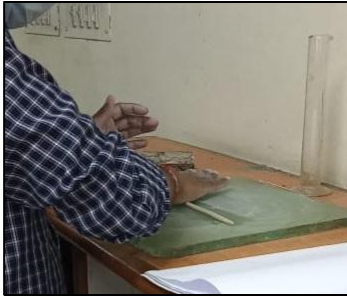
Fig.4.11: Performing plastic limit (DTU)
