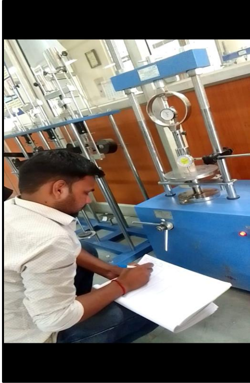
Fig.4.15: Performing UCS test
