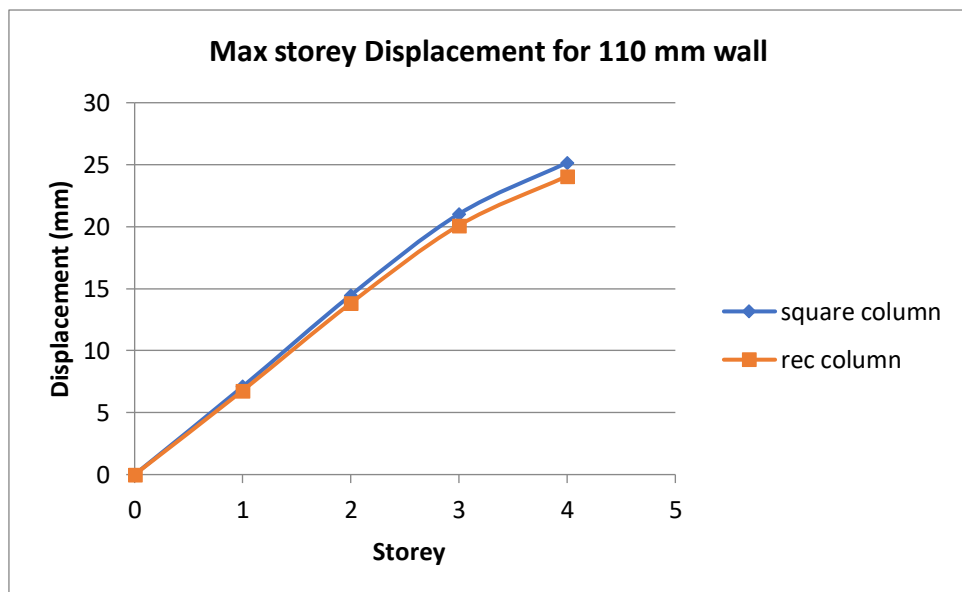
Fig.4.39 Max storey displacement for square & rec. column in Y-Dr (wall model as CDS)
