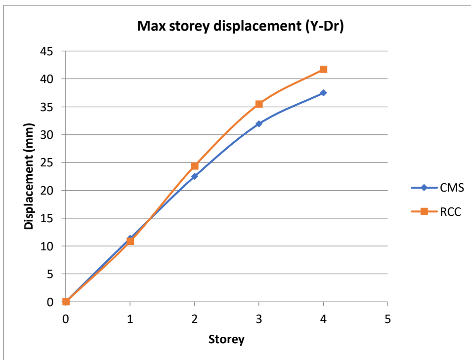
Fig.4.2 max storey displacement for CMS & RC frame structure in Y-Dr
