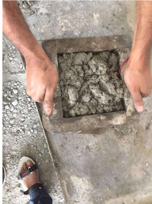
Figure 3.2. Mould filled with concrete
