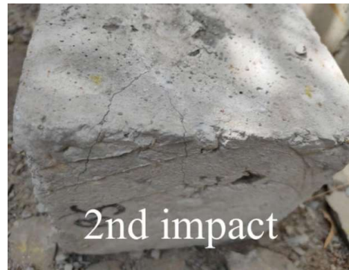
Figure 4.24 cracks widening after 2 nd impact
