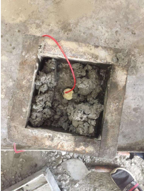
Figure 3.1 PZT- placed in centre of the cube
