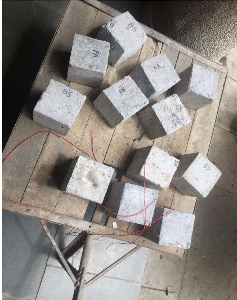
Figure 3.3. Concrete cubes with PZT embedded demoulded after 24 hr
