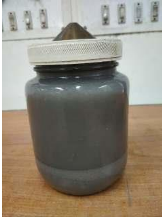
Figure 4.2: Specific gravity determination through Pycnometer
