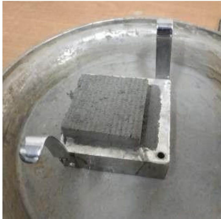
Figure 4.4: Failed specimen in Direct Shear Test
