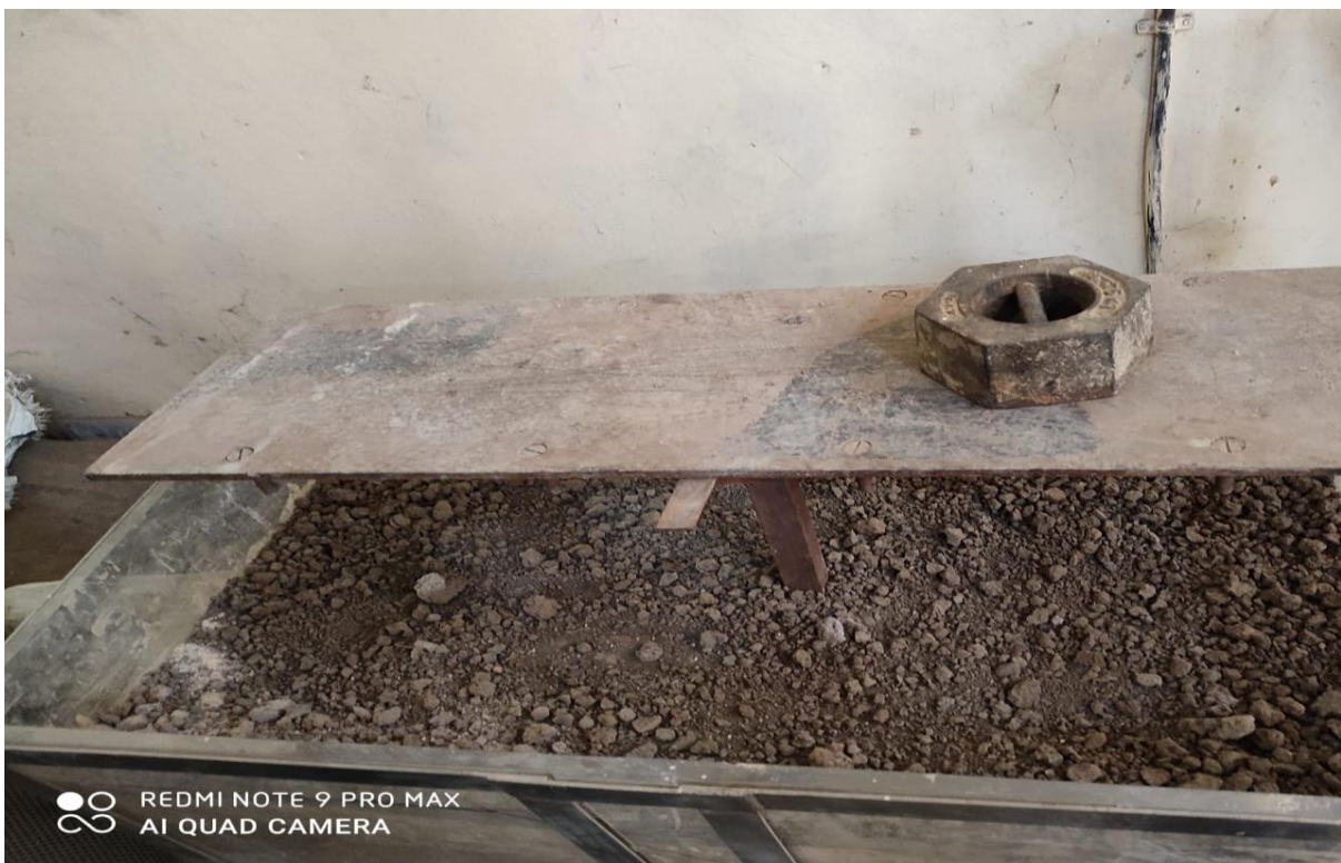
Figure 3.5: Eccentric loading on footing
