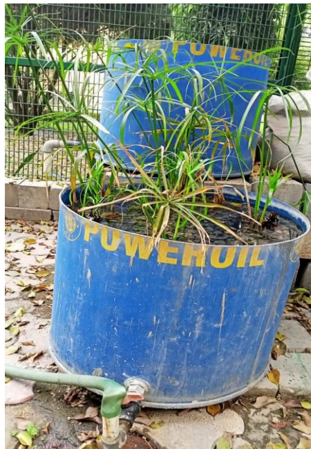
Fig. 2.2 Cyperus alternifolius based CW used during the study.
