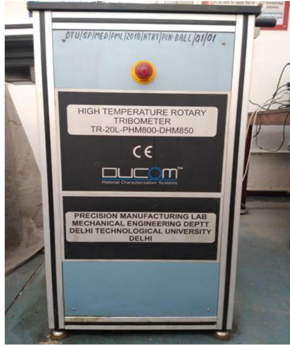
Fig 1.4 :- Experimental Setup For Pin On Disc Wear Experiment
