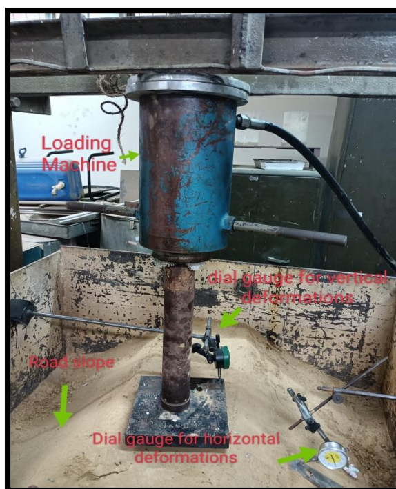
Fig.4.6 Loading machine along with the dial gauges
