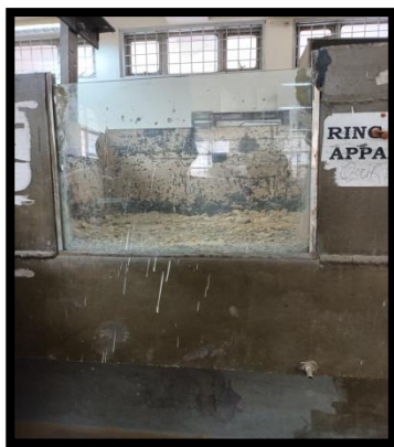
Fig. 4.7 Rectangular tank used for physical modelling
