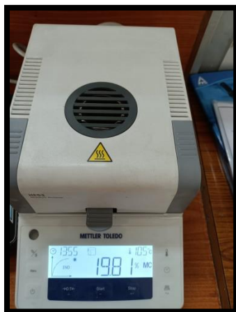
Fig. 3.4 Moisture meter showing water content
