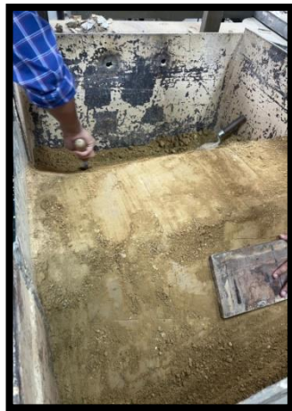
Fig. 4.1 Preparation of unreinforced embankment
