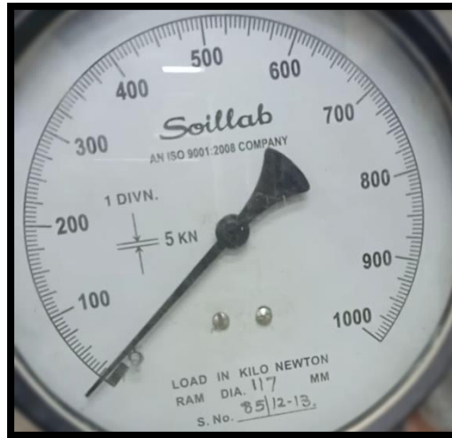
Fig. 6.8 Proving ring showing failure load for single layer reinforced slope
