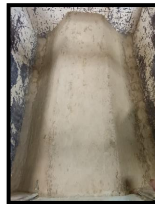
Fig. 4.4 Slope with a single layer of reinforcement
