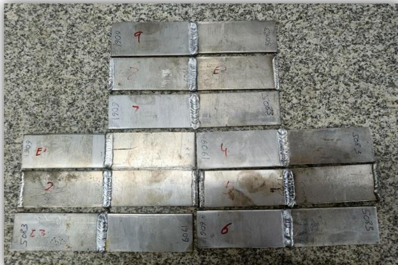
Fig19: GTAW welded plates
