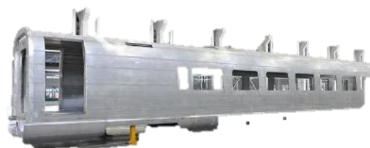
Fig3: Aluminium coach frames used in metros and LHB coaches. (MCF Indian railways)
