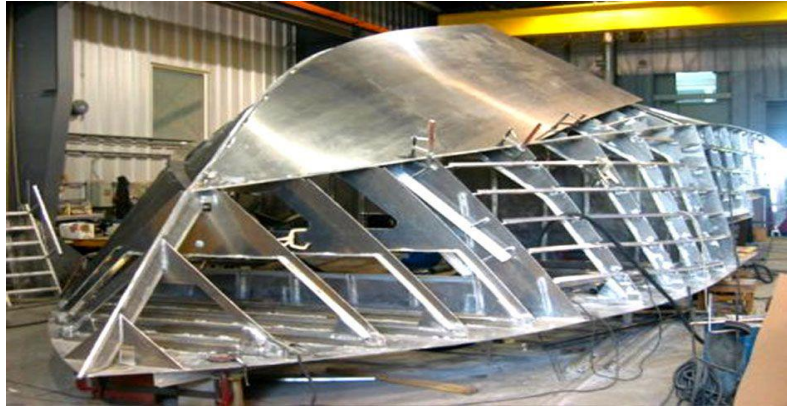
Fig7: frames and body panes of yacht. (Coenen yachts America)
