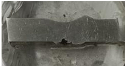
Fig18: Weld bead at deferent welding current
