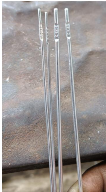
Fig13: ER4043, ER4047, ER5356 filler rods.
