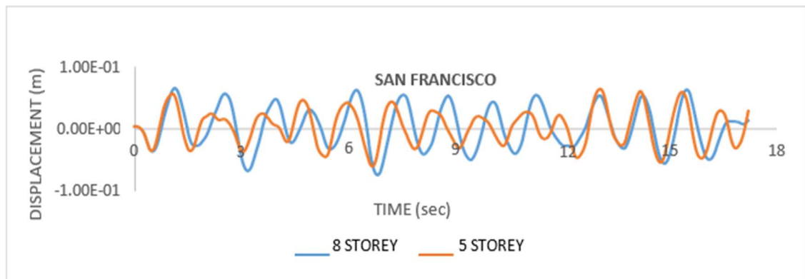
FIGURE 5.5 Displacement vs time graphs of SMGMs used (Y direction-bare frame).
