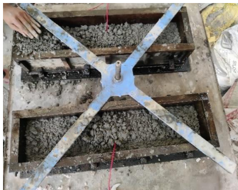
Fig. 3.5 Placing the PZT patch in the concrete
