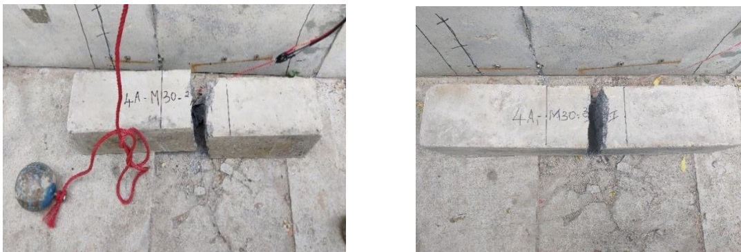
Fig. 4.3 Crack due to impact height of 3m and 2.5 m respectively
