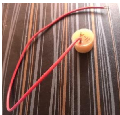
Fig.3.4. PZT patch covered with epoxy
