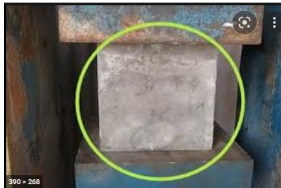
Fig 4.9. M20 Cube load application
