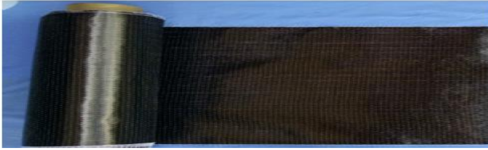
Fig 4.3. used CFRP “Sika CarboDur S”
