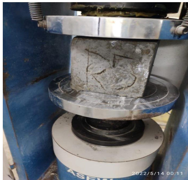
Figure 29: CTM testing for R5 cube (II)
