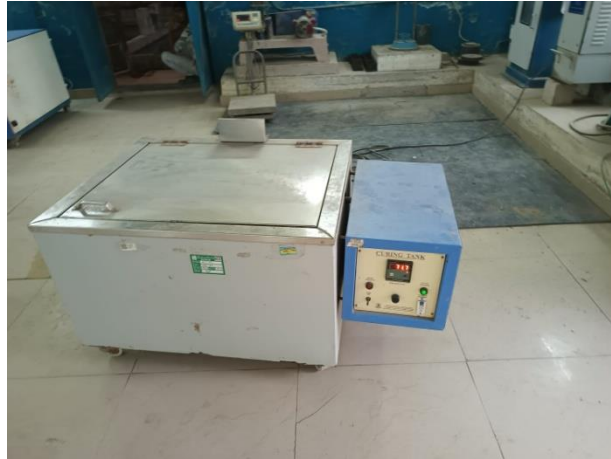
Figure 21: Accelerated Curing Tank
