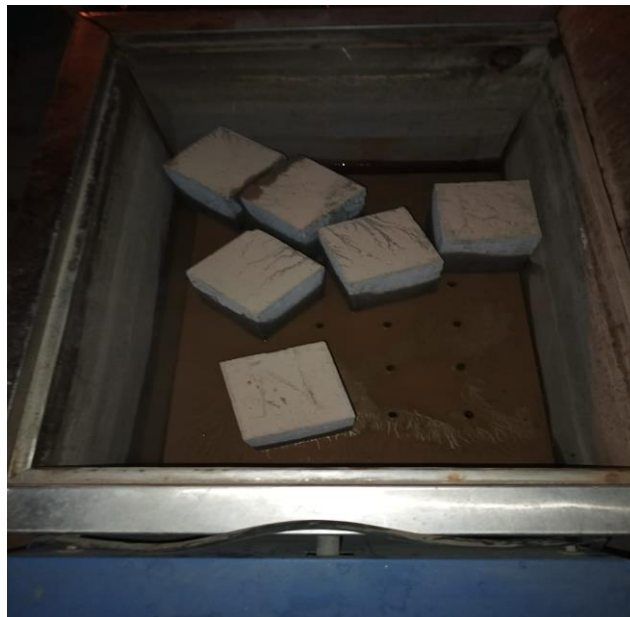
Figure 22: Cubes under the process of curing
