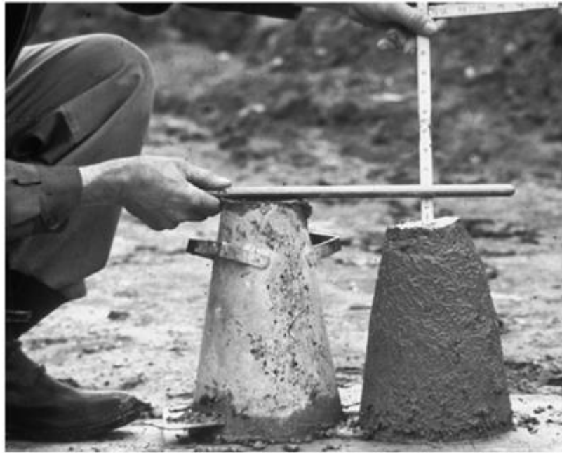
Figure 2: Concrete slump test with a slump of 1.5 in., typical for pavement work. (Portland Cement Association) [1]
