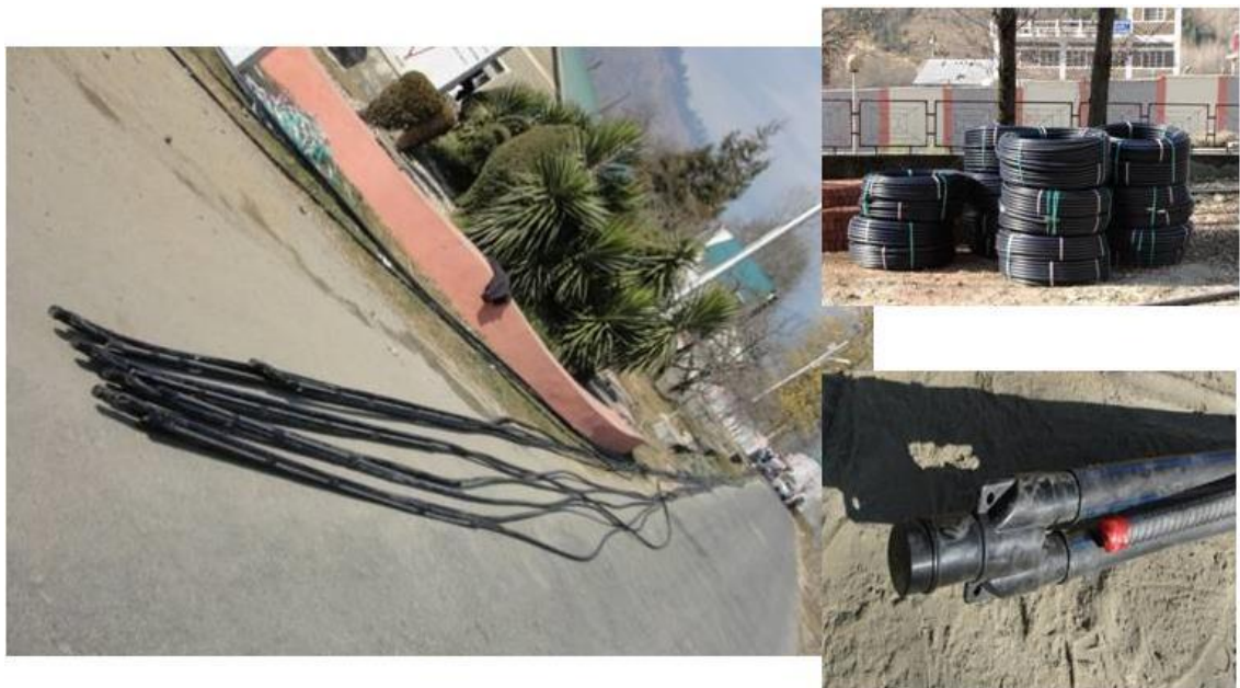
Figure 3.4: HDPE U-bent for vertical boreholes installation, top view is the roll of HDPE pipes (U-bent) and bottom view is the end of U-bent.
