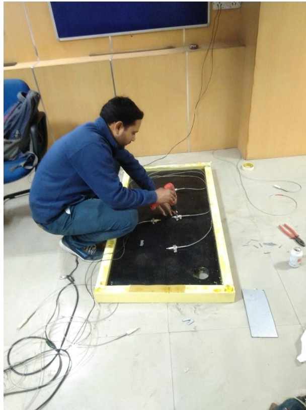
Figure 4.1.2: Installing the thermocouple on absorber plate
