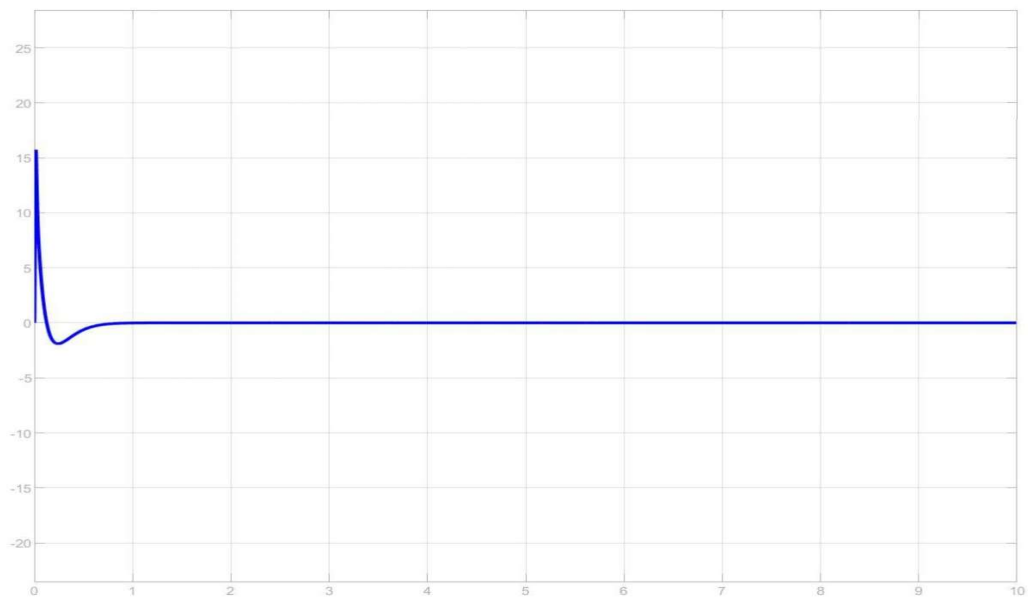
Figure 6.5 Angle disturbance with MATLAB autotuner PID parameters
