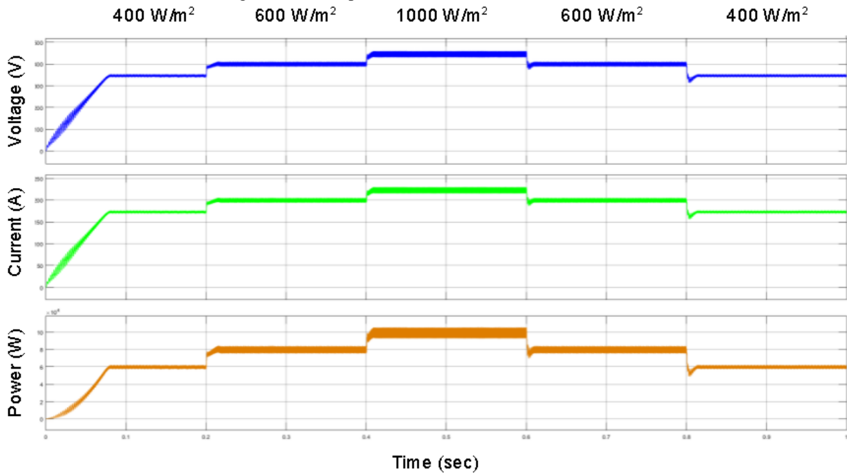
Fig 6.6 CBC Output waveforms at 25^\circ\text{C} temperature with different irradiation
