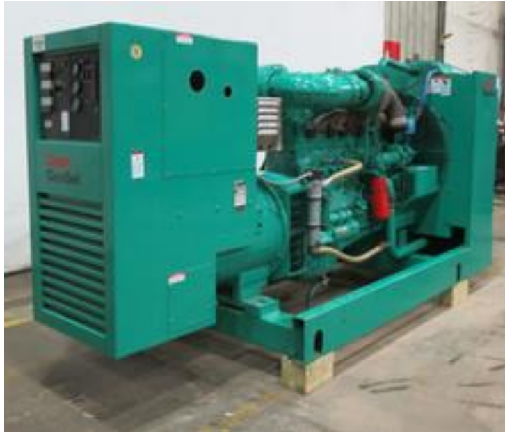
Figure 4.1 - An Average 250 Kw diesel generator.
