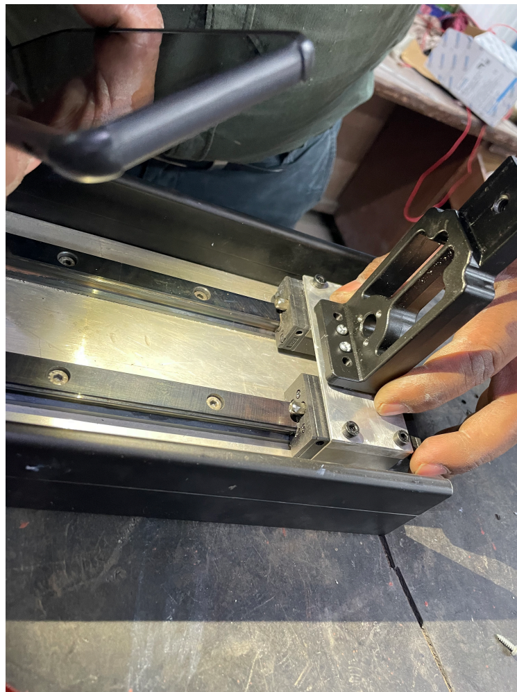
FIG 7.1:- DEPICTS MECHANICAL ASSEMBLY OF DUAL Z-AXIS
