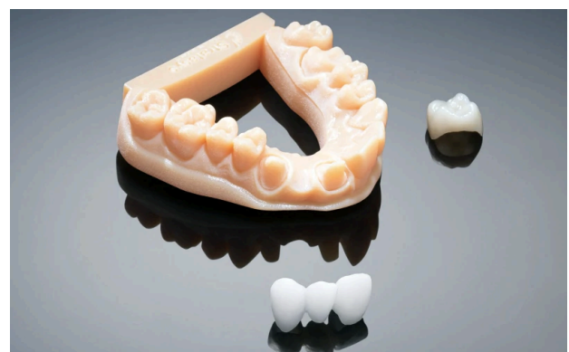
FIG 3.5: 3D PRINTED TEETH
