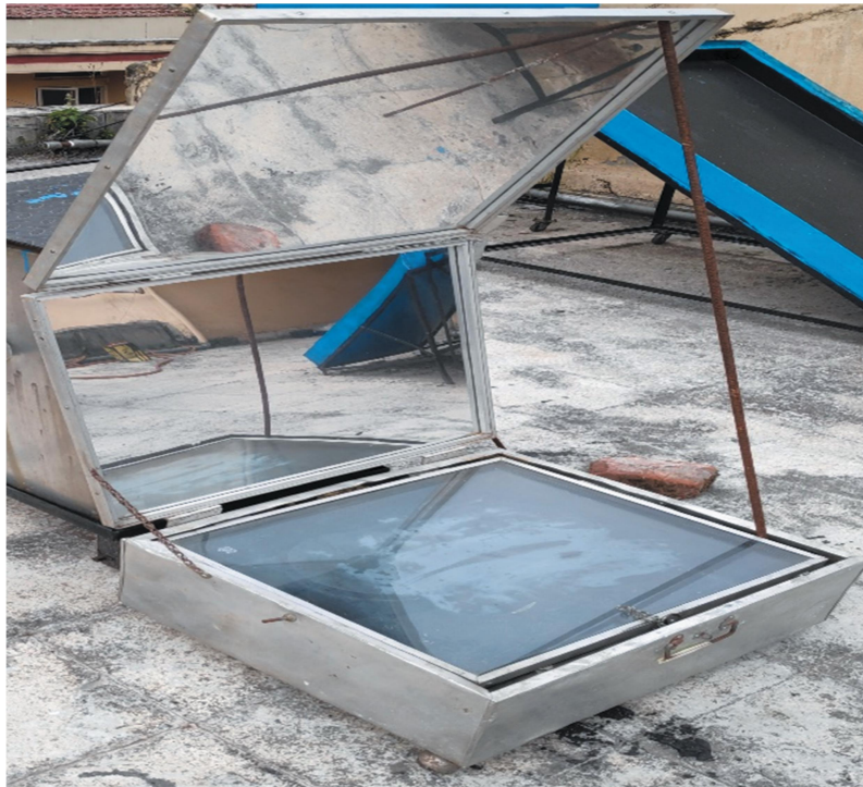
Fig 2.2: Photograph of double reflector box-type solar cooker
