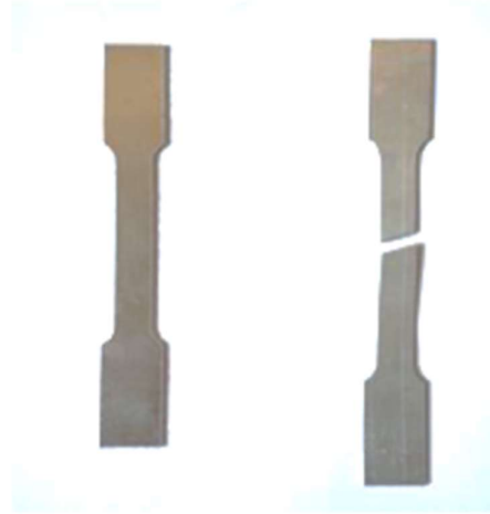
Figure.14: Specimen before and after the tensile test
