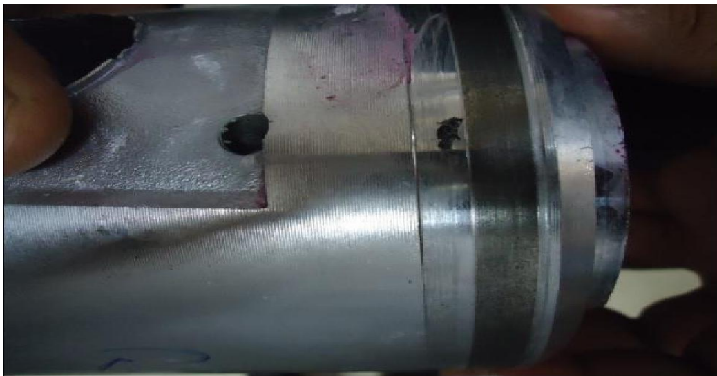
Figure- 3.5 Shift Defect in Piston.
