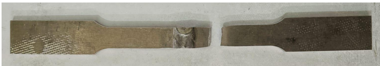
Figure 4.11: Fractured weld specimen E8 of ER5356
