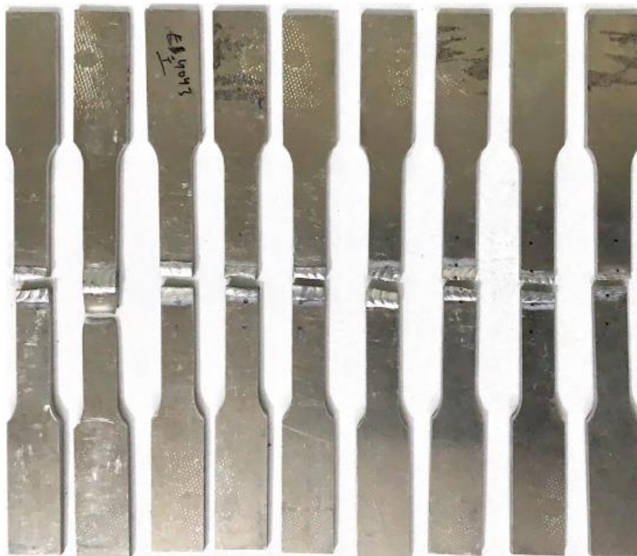
Figure 4.4: fractured welded samples of ER4043
