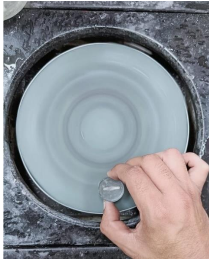
Figure 3.13: Polishing of sample by emery paper
