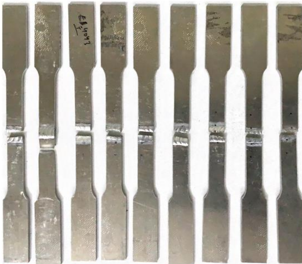
Figure 4.7: fractured welded samples of ER4047
