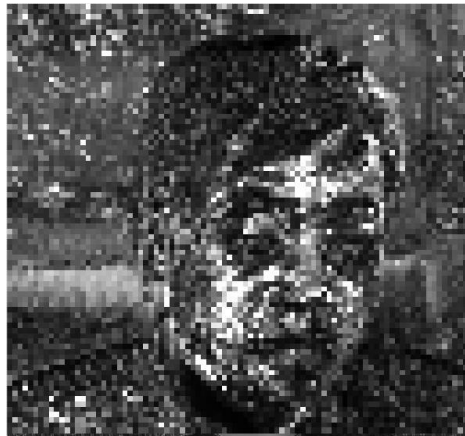
Figure 5.3: Pulse Amplitude Map at Heart rate frequency with 10x10 grid size
