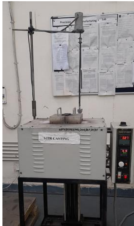
Fig 3.3: Stir Casting setup
