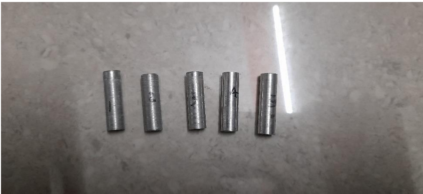
Fig 3.5: Sample specimen of wear test
