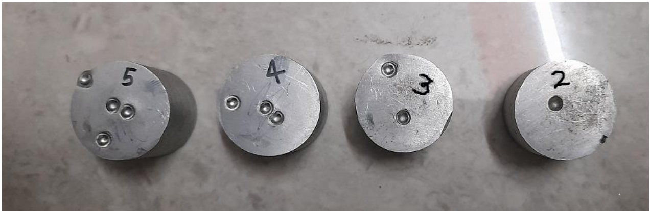
Fig 3.5: Tested samples of brinell hardness test
