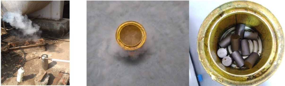
Fig 4.9.3 Sequence from collection of liquid nitrogen to performing cryogenic soaking to obtaining alloy pieces after cryogenic soaking
