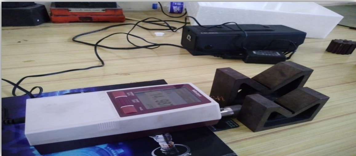
Fig 3.3.3.1 Surface roughness measurement using Mitutoyo surfest SJ210 series
