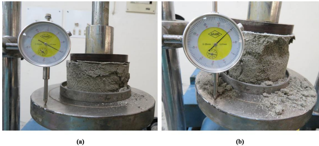
Figure 5.8 Failure mode of the sheared specimens under axial loading during UCS testing (a) C 1 column; and (b) C 2 column
