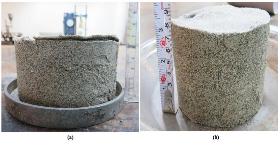
Figure 5.6 Treated specimens for UCS testing (a) C 1 column; and (b) C 2 column
