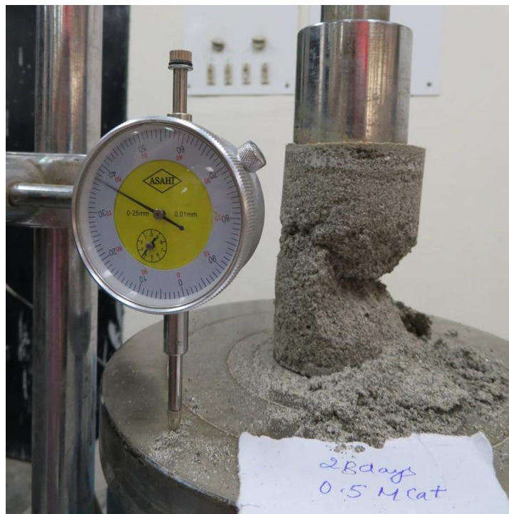
Figure 3.9 Shear failure in the 28 days specimen (set I) during the UCS testing
