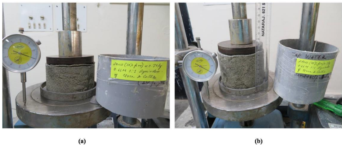
Figure 5.7 (a) Mount C 1 column; and (b) Mount C 2 column to apply the axial load
