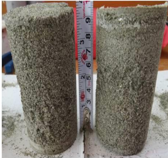
Figure 3.8 (a) The 14 days biotreated sand column for UCS testing
