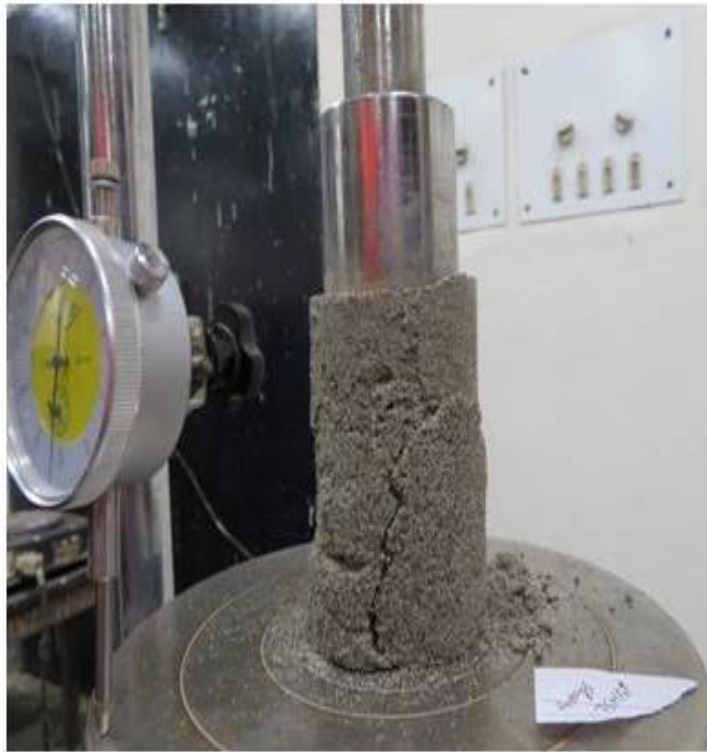
Figure 3.8 (c) Shear failure propagation in the 28 days biotreated specimen (set I)
