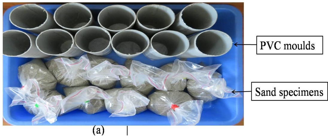
Figure 3.2 (a) PVC molds and sand specimens in polythene bags
