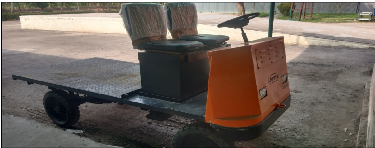
Fig 1.7: Electric Trolley for Transportation of Goods with-in Industries
