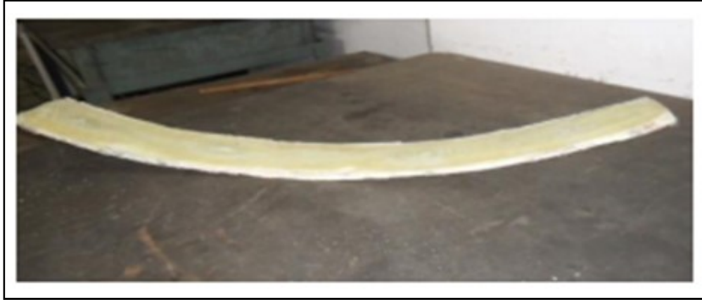
Fig.1.6: Prototype of composite leaf spring (Venkatesan and Devaraj, 2012)
