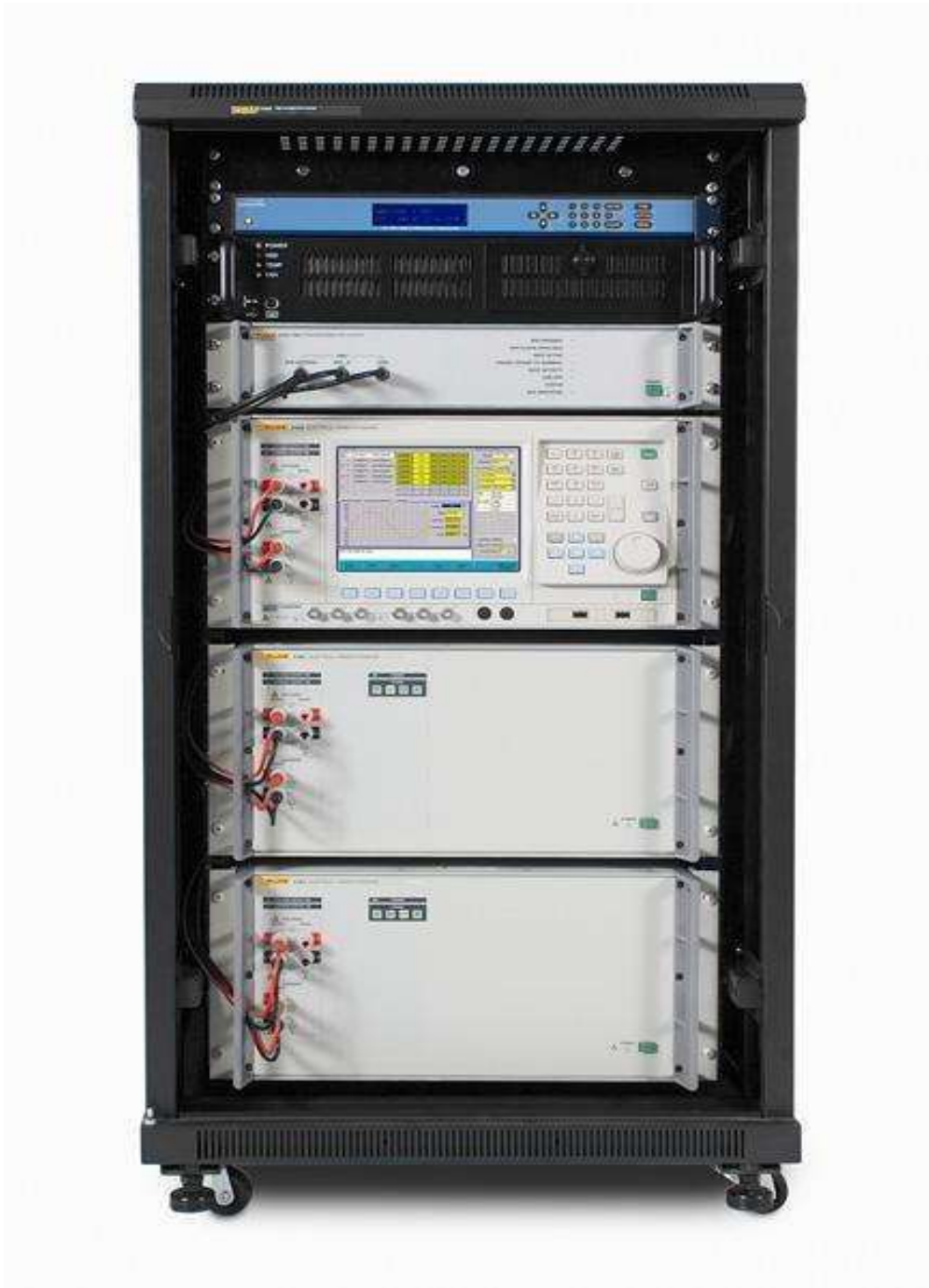
Fig.1.8 Station Phasor Measurement Unit
