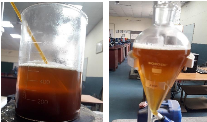
Fig. 4 – Jatropha Biodiesel prepared at Lab. for Testing
