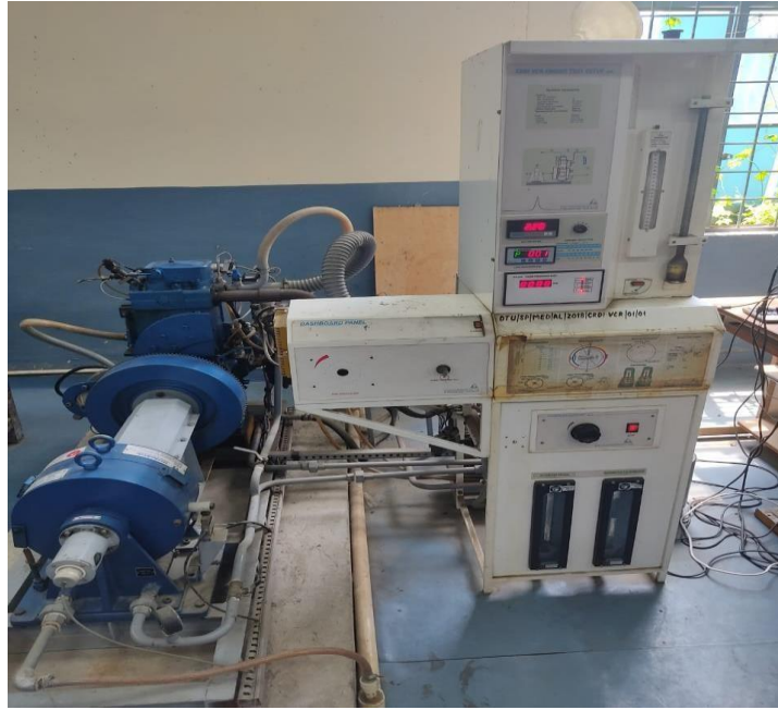
Fig. 5 – Kirloskar Diesel Engine Test Setup
