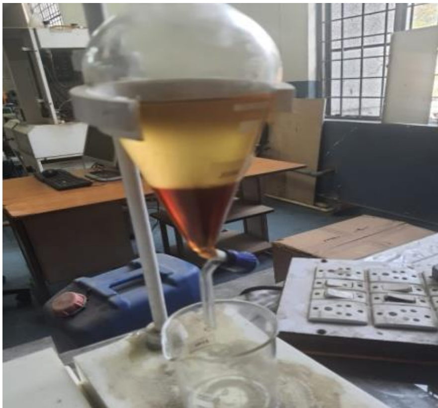
Fig. 3 Linseed Biodiesel prepared in lab.
