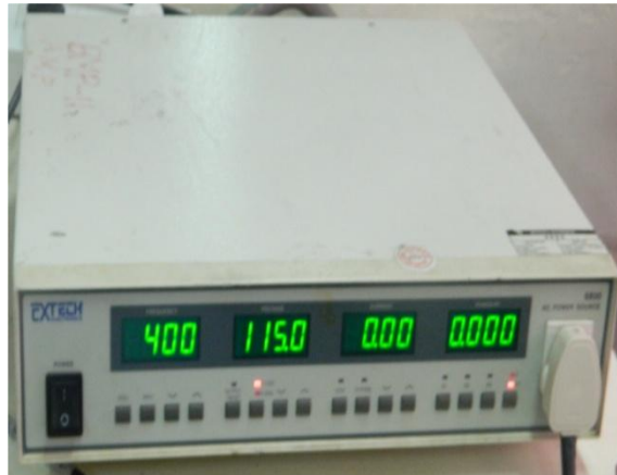
Fig.7.5 Reference Supply Generator.
