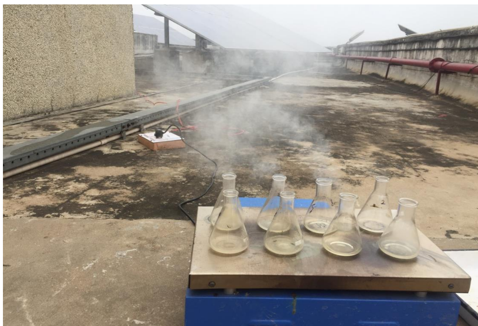
Fig 3.8: Acid Digestion of Dust samples on Hot Plate
