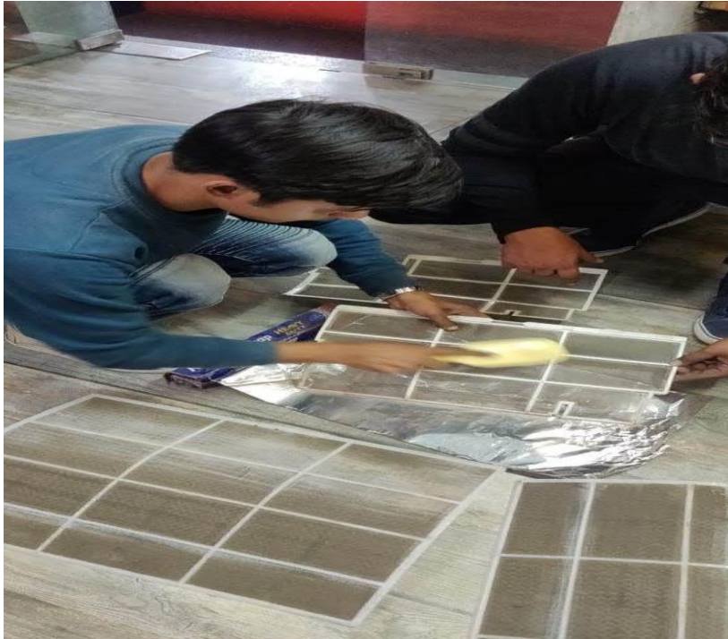
Fig 3.3: Dust sample collection with the help of Brush
