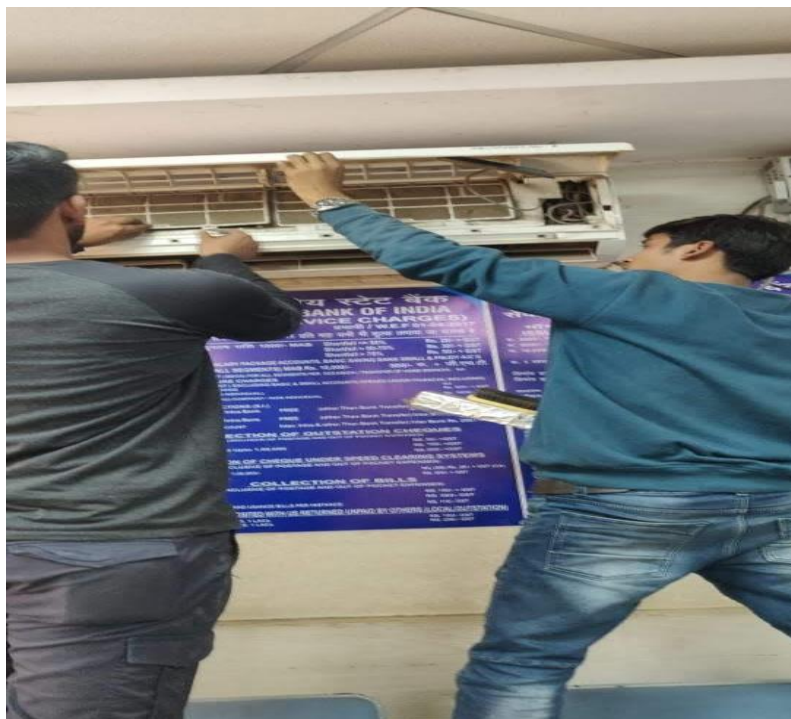
Fig 3.4: Extraction of dust sample from AC filter.
