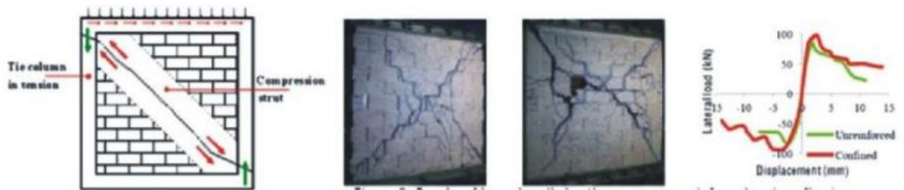
Figure 8: cracking Behaviour of confined masonry
