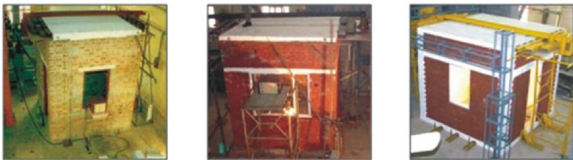
Figure 9: Single Storey model of Unreinforced, reinforced and confined masonry for experiment by Chourasia.et.al
