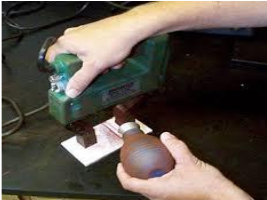
Fig.3.6 Magnetic particle inspection [15]
