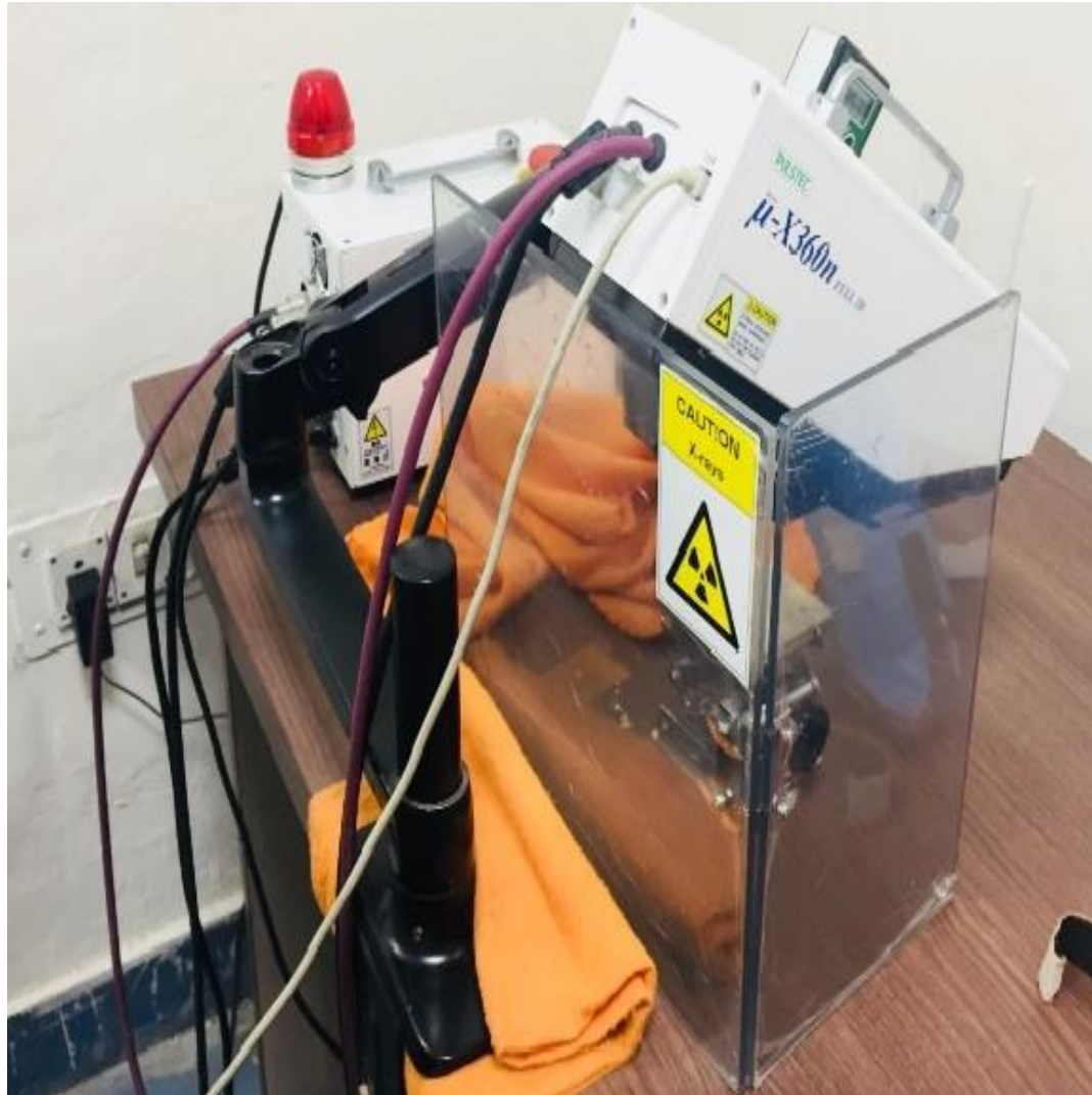
Fig.4.11. \mu -X360s X-ray residual stress analyser
