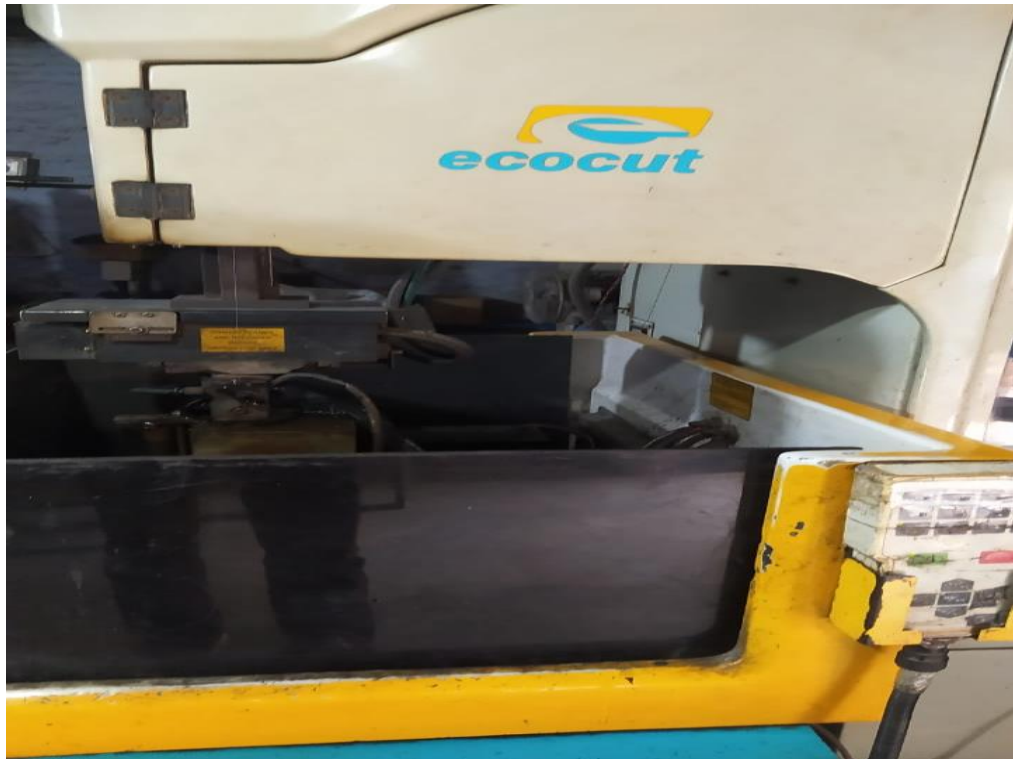
Fig.4.4 EDM Wire Cutting under Process.
