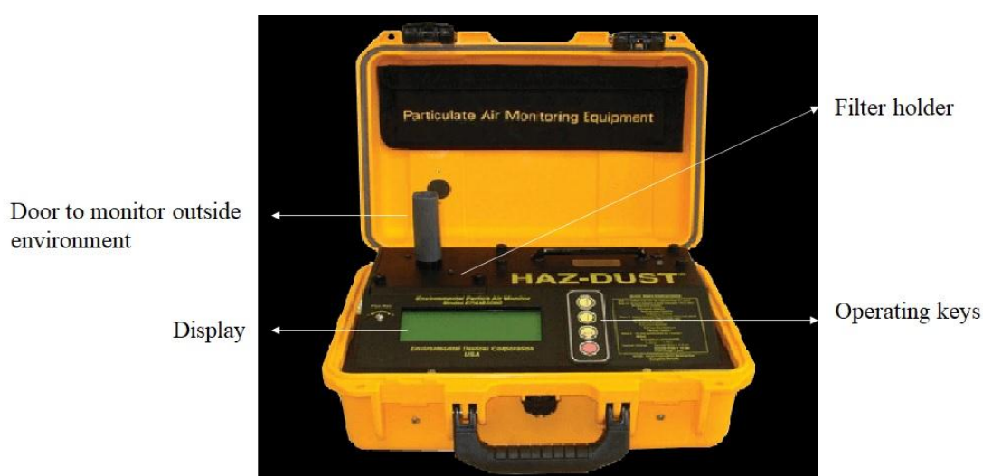
Fig 3.6 HAZ DUST EPAM 5000 instrument used for RSPM test
