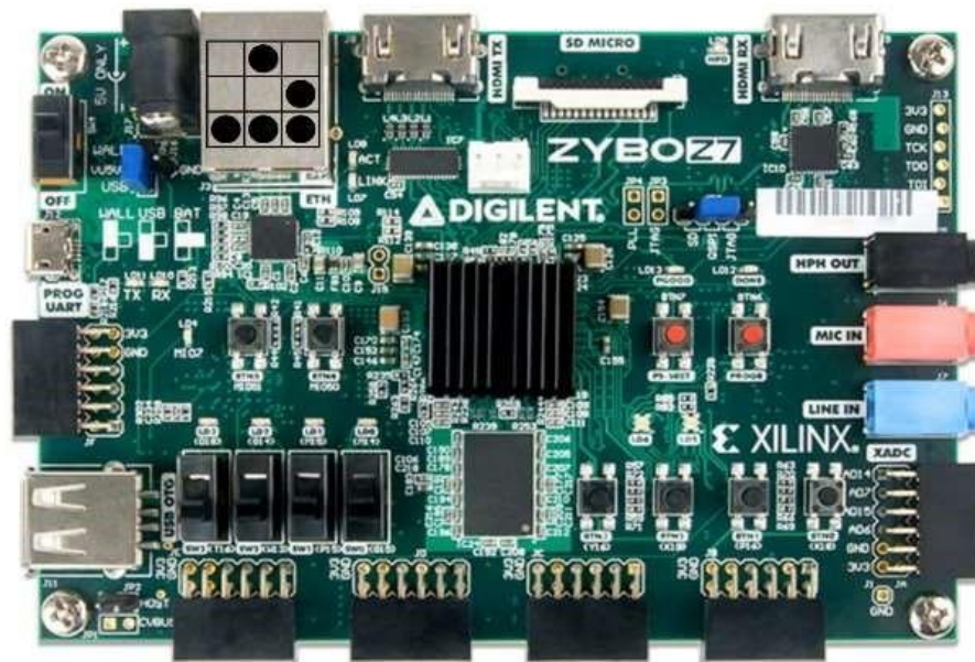
Figure 3.8 ZYNQ 7000 FPGA board [30]
