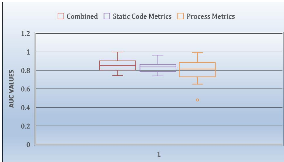
Fig 6.19 Box plots of combined model, model solely containing static code metrics and model solely containing process metrics using voting
