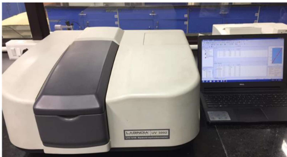
Fig. 3.4 Double beam UV-Vis Spectrophotometer (Lab India make UV 3092 model) used for determining the catabolic enzymatic activities
