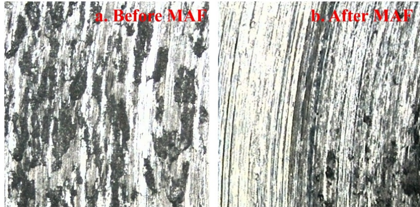
Figure 8.1 Micrographs of Ti-6Al-4V surface before and after magnetic abrasive finishing.
