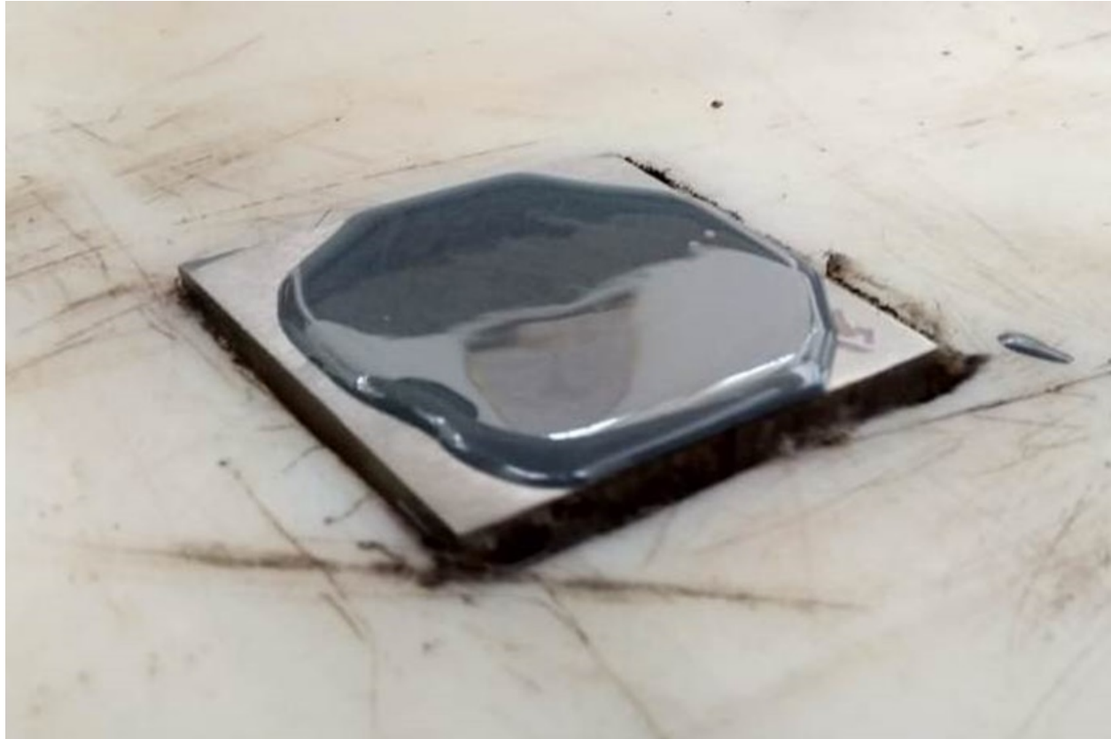
Figure 6.7 Media on the workpiece in the absence of magnetic field.
