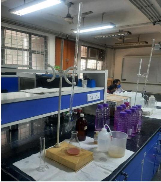
Figure 4 titration method for determination of alkalinity
