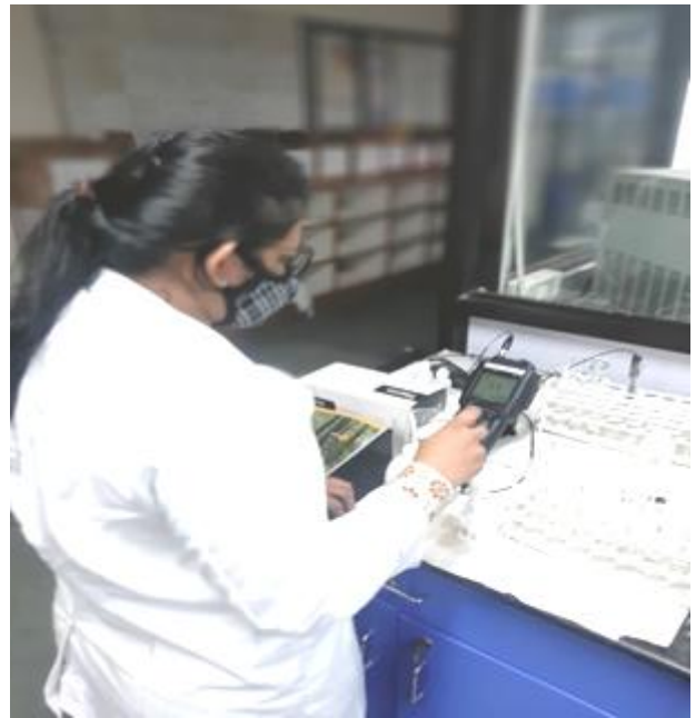
Figure 2 Ion specific F meter (Orion make star 320 model) used for analysis
