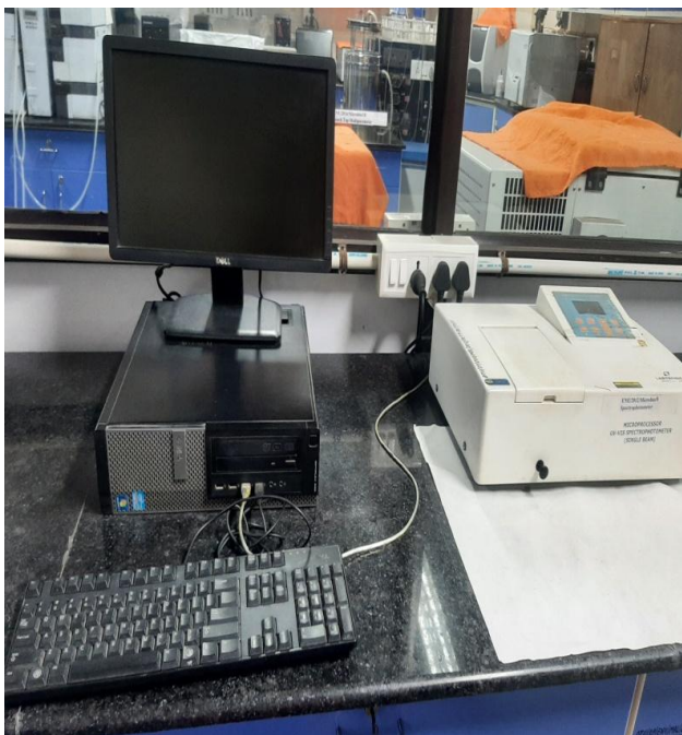
Figure 3 , Spectrophotometer analysis (, Labtronics model-LT-290 ) for determination of chemical characteristics of water
