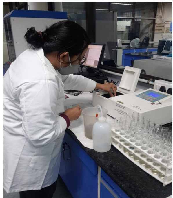
Figure 3 , Spectrophotometer analysis (, Labtronics model-LT-290 ) for determination of chemical characteristics of water
