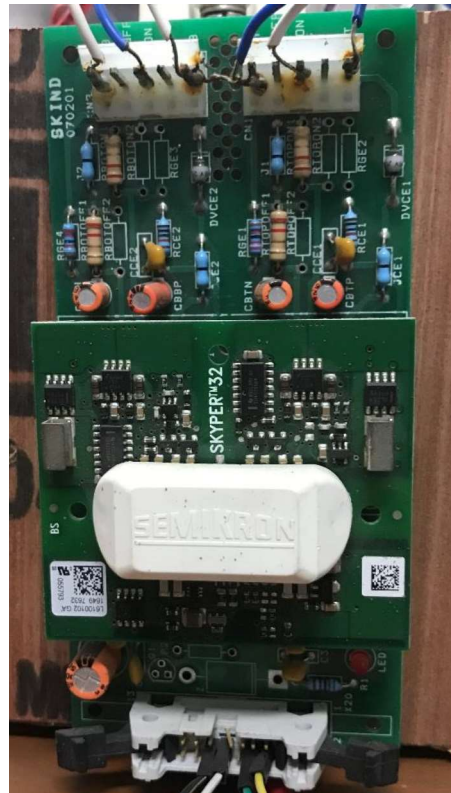
Figure 2.20: Gate driver circuit.
